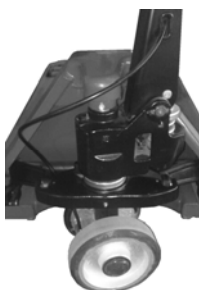
Fig.12: Progressive drive and parking brake
